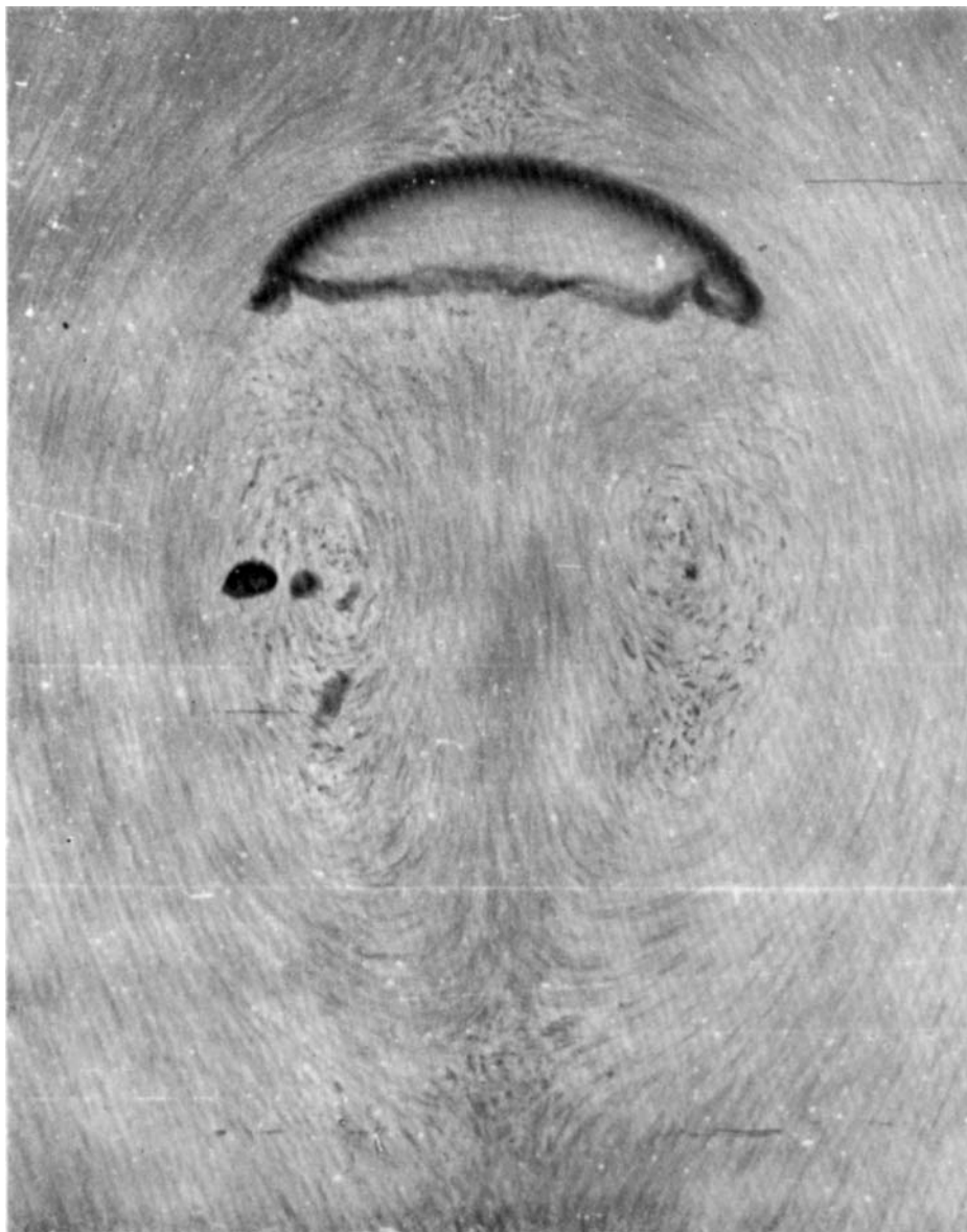
FIGURE 2. Wake structure for a large two-dimensional gas bubble.
